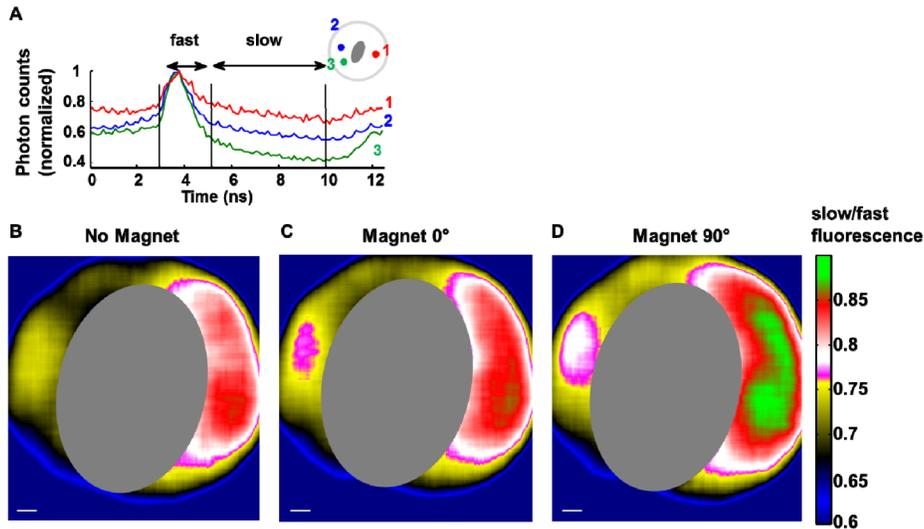
Fig. 4. MFE mapped with 2-photon-excited time correlated single photon counting. A) Histogram of arrival times relative to the excitation pulse at  $t = 4$  ns for three locations around the wire with different magnetic field strengths. B-D) Images of the ratio of slow to fast fluorescence counts. This ratio reports local magnetic field without need for a reference image. Scale bars 10  $\mu\text{m}$ .
