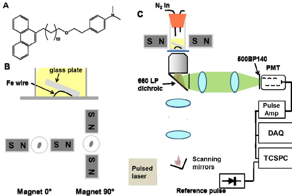
Fig. 1. Apparatus for 2-photon magnetic field imaging. A) Magneto-fluorescent indicator, Phen-12-O-2-DMA. B) Sample geometry. Top: side view of the sample chamber. The glass plate ensured that the Fe wire did not move in the applied magnetic field. Bottom: top view of the sample chamber showing the arrangement of the permanent magnets and the elliptical cross-section of the Fe wire in the center of the chamber. C) Two-photon imaging apparatus. Abbreviations explained in the main text.
