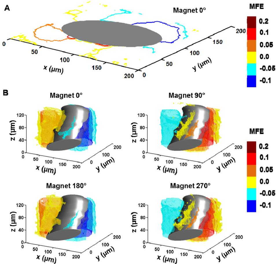
Fig. 3. 3D mapping of MFE around an iron wire. A) Contours of MFE strength in a slice imaged around the Fe wire at  $z = 50 \mu\text{m}$ . B) 3-dimensional mapping of the MFE around a section of Fe wire. Contours represent surfaces of constant MFE strength. Images were acquired with  $\delta z = 10 \mu\text{m}$  between sections, and  $500 \text{ nm}$  in-plane spatial resolution.
